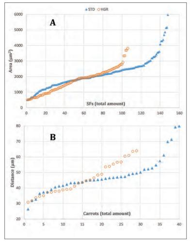
Figure 6. Moving from a standard growth rate process (STD) to a high growth rate process (HGR) reduces stacking faults (A) and carrots (B) in the epilayers.
