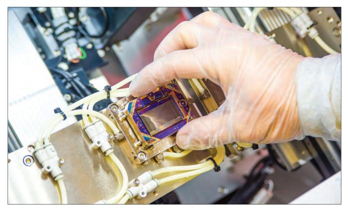
The foundry at CST Global includes an automatic bar stacker.
