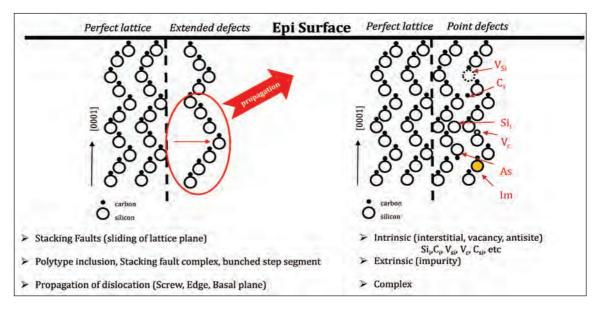
ensures uniformity, in terms of thickness and doping. A greater challenge is the realisation of a low defect density in the epilayers.
