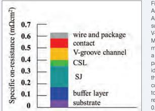
Figure 2. Analysis of AIST's SiC super-junction V-groove MOSFET, mounted in a TO-268 package, identified the primary contributions to a total onresistance of 0.63 mΩ cm<sup>2</sup>.
