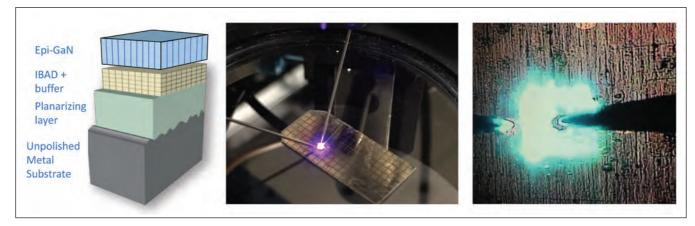
Figure 1. iBeam Materials' GaN-on-metal technology relies on a single-crystal-like layer that is created on top of a polycrystalline substrate, such as a long-length metal foil. The single-crystal-like layer is formed by an ion-beam-assisted deposition process. On the left is shown the layer architecture, while photographs show the first LED devices.
