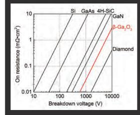
Theoretical specific on-resistance as a function of breakdown voltage. The solid lines indicate the theoretical limit, determined from the material properties.
