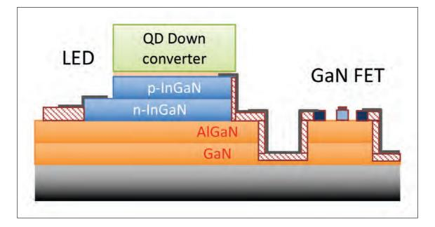
Figure 6. The sub-pixel LED can be integrated with an GaN/AIGaN FET transistor device, by integrating the FET in the epi structure.
