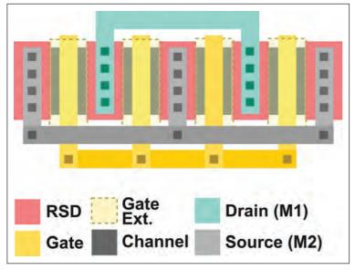
Figure 2. The layout of IBM's RF-MOSFET with four gate fingers. The gate extension layer indicates an additional metal line on top of the gate metal to reduce the gate resistance.
