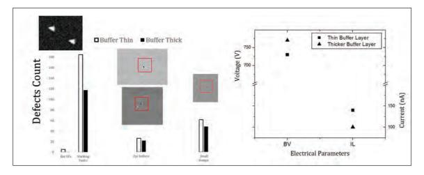
Figure 5. Thicker buffers reduce the defect densities in the epilayer (left), and improve the performance of the MOSFET (right), which benefits from a higher breakdown voltage and a reduction in leakage current.
