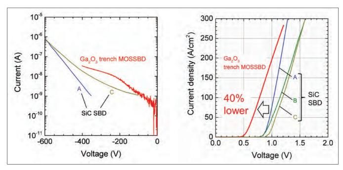
Figure 3. (a) Reverse and (b) forward characteristics of a  $\beta$ -Ga<sub>2</sub>O<sub>3</sub> trench metal-oxide-semiconductor Schottky barrier diode and a commercially available SiC Schottky barrier diode. The  $\beta$ -Ga<sub>2</sub>O<sub>3</sub> device exhibits about a 40 percent lower forward loss than that of the SiC Schottky barrier diode, and has small reverse-leakage characteristics.
