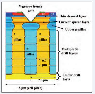
Figure 1. AIST's SiC super-junction V-groove MOSFET is claimed to set a new benchmark for on-resistance for SiC MOSFETs with a blocking voltage in excess of 600 V. The device combines a blocking voltage of 1170 V with an on-resistance of just 0.63 m $\Omega$  cm².
