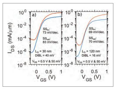
Figure 3. Subthreshold characteristics for short and long-channel finFETs for logic applications. The tri-gate architecture of the finFET improves electrostatic control to reduce the off-current at the intended bias point.
