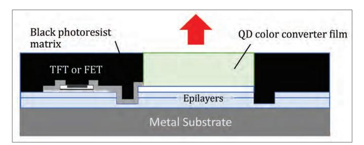
Figure 5. A sub-pixel cross-section showing a quantumdot, colourconverting film and black photoresist matrix.
