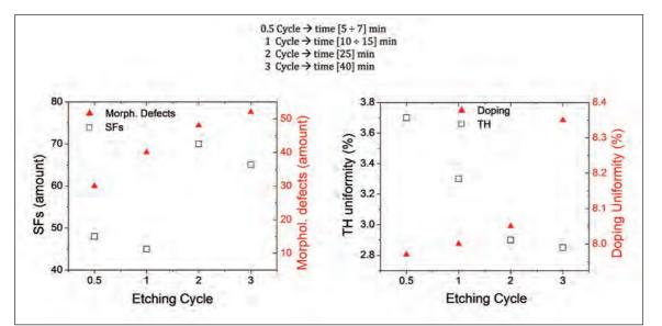
Figure 4. (Left) The number of defects as a function of etching time. (Right) Thickness and doping uniformity as a function of etching time.
