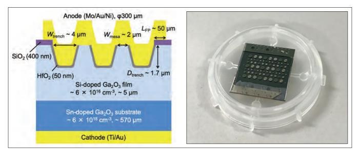
Figure 2. The β-Ga<sub>2</sub>O<sub>3</sub> trench metal-oxide-semiconductor Schottky barrier diode developed by Novel Crystal Technology and Tamura Corporation.
