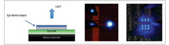
Figure 2. Diagram of an LED cross section, and emission from a 20  $\mu$ m blue LED on metal and an array of microLEDs
