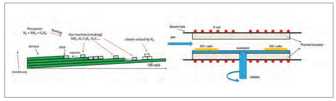
Figure 1. (left) Decomposition of precursors on the substrate surface, followed by migration of atoms, leads to 4H-SiC homoepitaxy growth. (right) Growth of SiC epiwafers is most commonly undertaken in a horizontal hot-wall CVD reactor.
